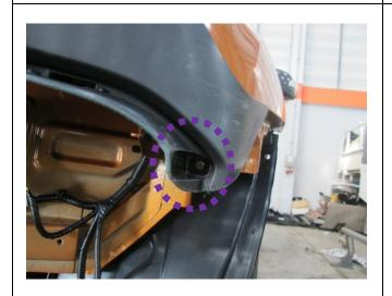
☐ Mount the bumper with the bracket using the M6 bolt provided in the bolt kit.
