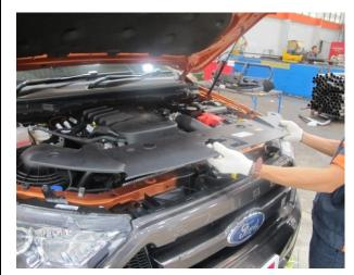
☐ Undo scrivets and take off the top radiator shroud and retain it.
