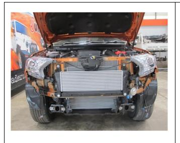
☐ Frontal view after removal of air dam and cross beam.
