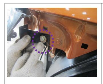
☐ Mount the bracket at indicated mounting point using the M6 bolt kit provided in the bolt kit.
