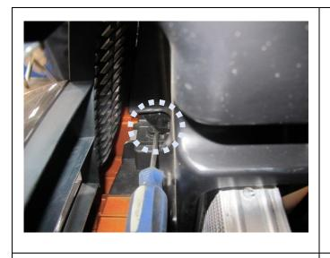
☐ Undo the indicated bolt and clip located behind radiator grill and discard it.
