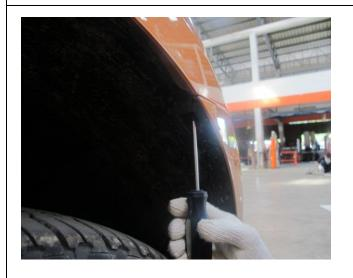
☐ Undo vertical screws in the wheel arch and retain.
