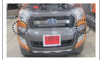
☐ Cut off original from the grill along the path and keep the indicated part for fastening.
