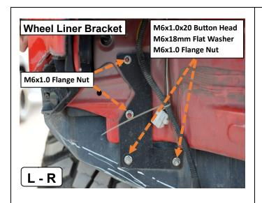
☐ Install wheel liner bracket provided in the fitting kit.
