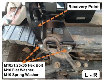
☐ Insert in the recovery point assembly provided in the fitting kit.
