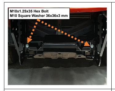
☐ Mount winch cradle (inner slot) using the supplied bolt kit.
