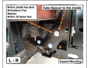
☐ Install support mounting with the provided bolt kit.
