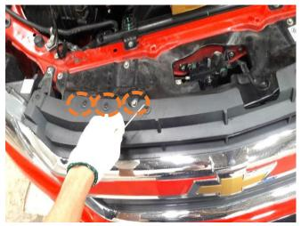
☐ Undo indicated (LHS & RHS) Allen screws and remove upper radiator shroud and retain.
