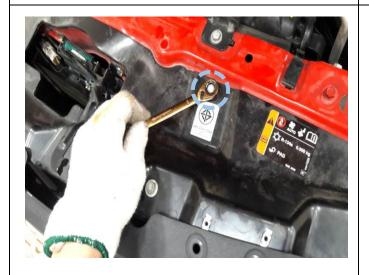
☐ Undo indicated bolt and remove lower radiator shroud and retain.
