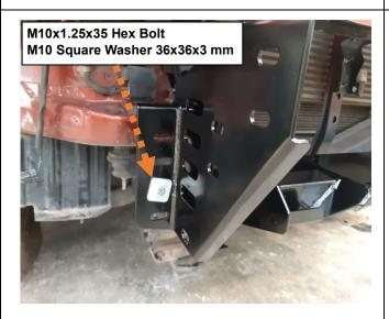
☐ Mount winch cradle (outer slot) using the supplied bolt kit.
