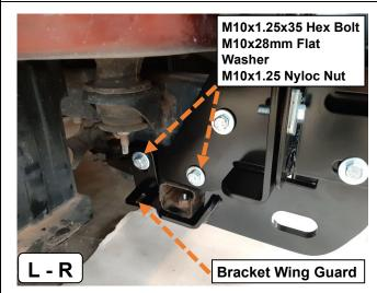
☐ Install wing guard bracket provided with the fitting kit.
